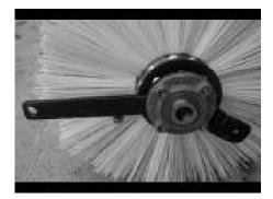
A self align bearing is fitted on the non-drive-side of the main broom. This must be greased periodically with lithium based grease. It is recommended that this bearing is checked for wear when the broom is removed for re-bristling and replaced if necessary.
