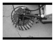
The Side Kerb Brush has a threaded adjustment stud fitted on the main support arm. This is adjusted according to brush wear. When the Kerb Brush is fully worn the three attachment bolts are removed and the complete brush head is replaced with a new brush head.
