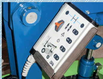
Wired remote control allows accurate placement of materials
